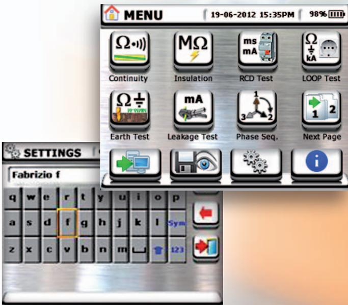
Adding a note and saving measurements has never been so easy thanks to its interactive keyboard.
